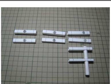
A photograph showing the completed gear frame assembly, consisting of several white frame components and the pipe, arranged on the grid background.                                      | 1) 各ギアを取り付けるためのフレームの完成です。                                         |
